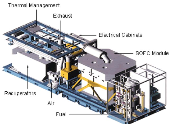
Fig. 8-1 : Major Components of a 100 kW SOFC Currently Operating in Hannover, formerly in Essen, Germany (Diagram courtesy of Siemens Westinghouse Power Corp.) [19]
