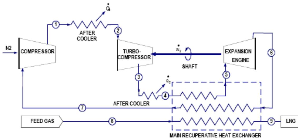
Fig. 5-1: Reverse Turbo-Brayton cycle refrigerator.
