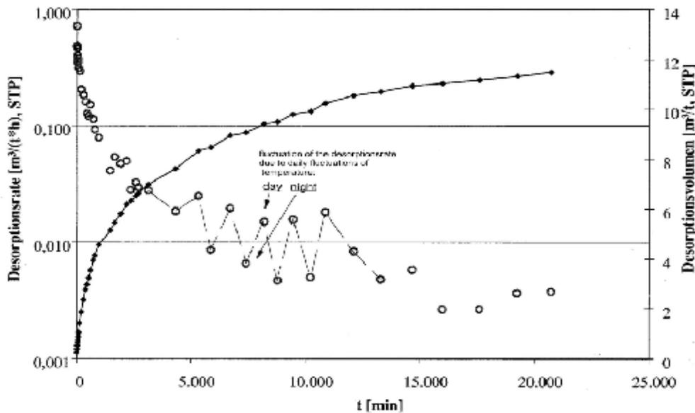
Fig. 1-3 Desorption of methane from a coal sample. [1]
