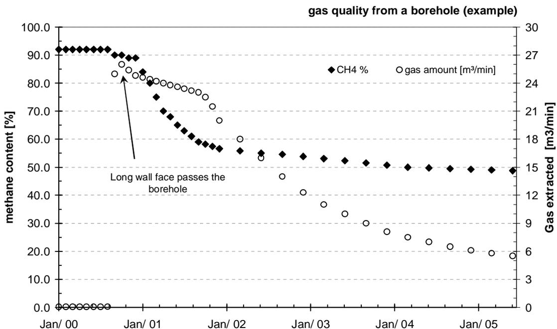
Fig. 1-2: Characteristic development of gas flow and CH<sub>4</sub>-content of CMM sucked at a borehole (source: Fraunhofer UMSICHT)
