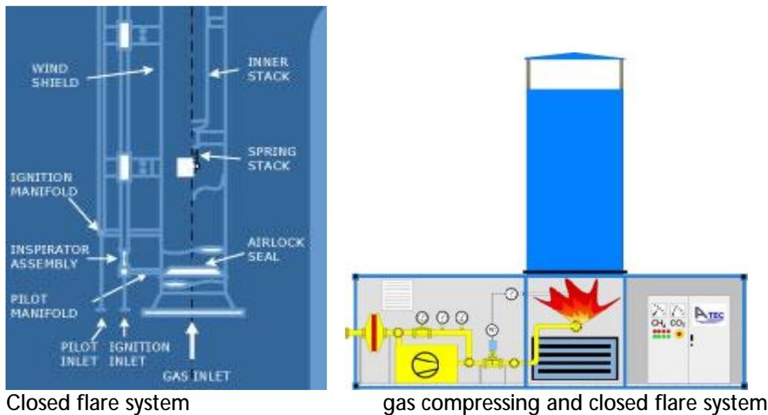
Fig. 4-2 : Major components of an enclosed flare system Source: A-TEC GmbH
