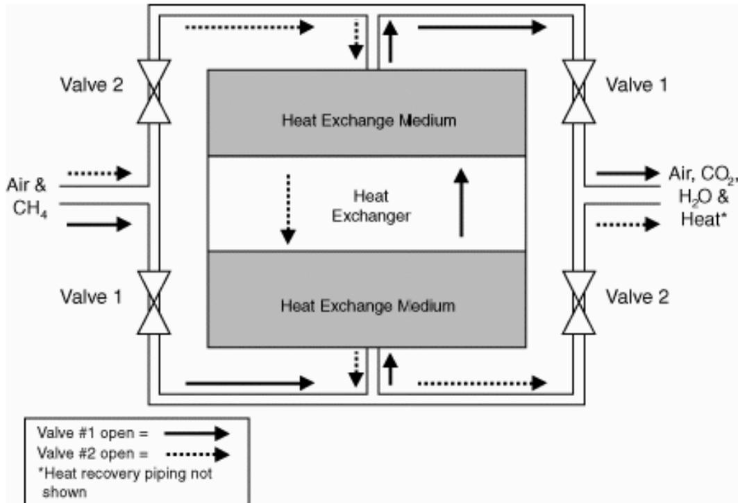
Fig. 6-1: Flow-Reversal Oxidation
